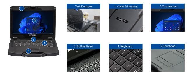
In order to test that devices would hold up to the sanitization procedure across their lifetime, it was completed 10,000 times at a pressure of 1kg/cm<sup>2</sup>.
